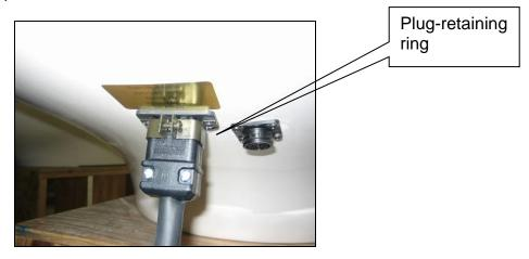
Figure 4.7.1 Connection of Power Cord
