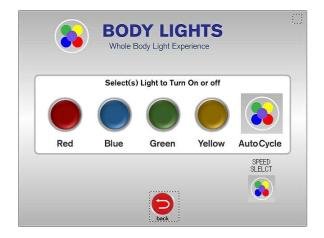
The AutoColor cycle speed can be modified by pressing the speed select key. The up/down will add or subtract 5 seconds. The AutoColor cycle is 5 second minimum to a 60 second maximum.
